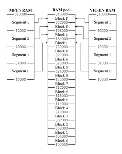
Figure 1: Memory mapping right after power-up
