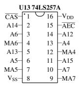
Figure 4: Pin-out for the multiplexer chip U13
