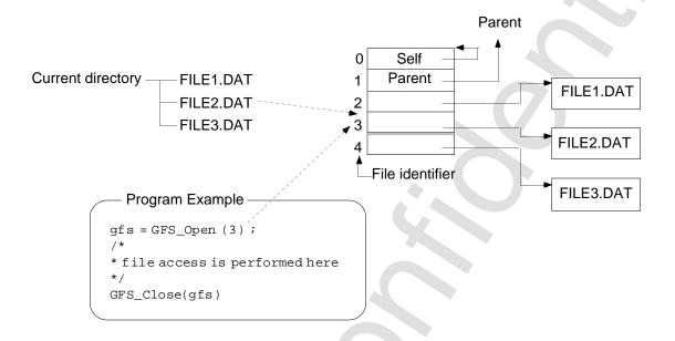
Figure 3.1 Access Using File Identifiers
