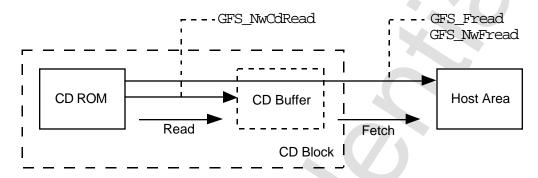
Figure 4.1 Access Function Model
