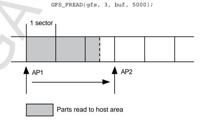
Figure 4.2 Movement of access pointer
