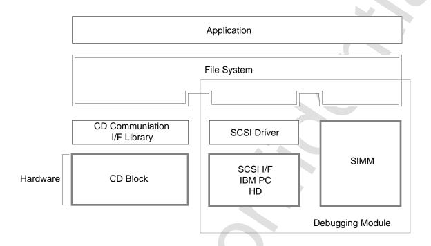
Figure 1.1 Module Configuration
