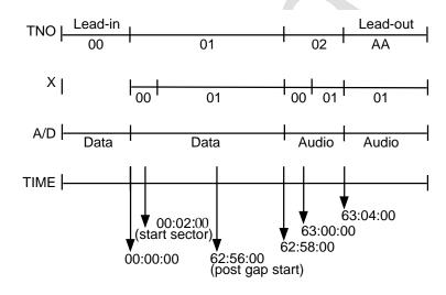
Figure 2.4 Track image when data track is maximized
