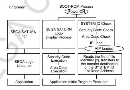
Figure 4.1 Overview from when the power is turned on
