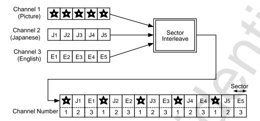
Figure 2.6 Sector Interleave by Channel Number
