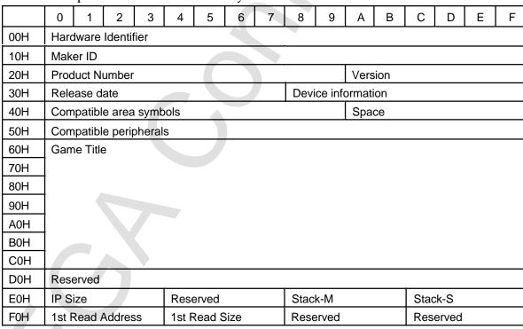
Figure 4.1 System ID Structure
