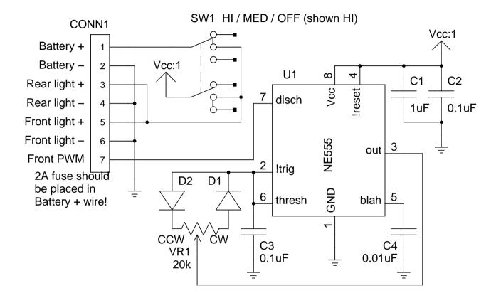
Bicycle LED headlight tunk: 555 oscillation frequency is about 600 Hz, duty cycle is adjusted by VR1. DISCH is used as output; it is open collector to GND as required by the LED driver. TITLE bicycle\_led\_dimmer.sch REVISION: 1.00 / 2020-12-04
