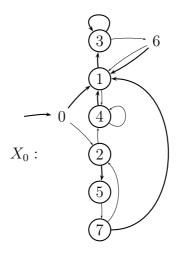
Figure 8: Automaton recognizing the language  $X_0$ , the first step of fixed point method
