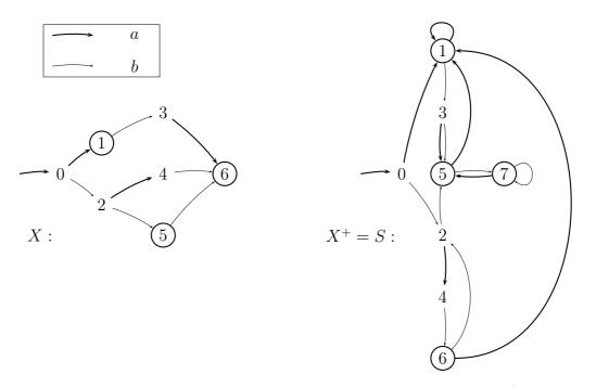
Figure 7: Finite automata recognizing languages X and  $X^+$ .
