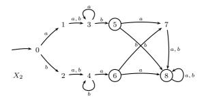
Figure 6: Automaton recognizing  $X_2$ . Computed with Grail+.
