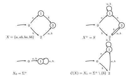
Figure 4: Minimized automata for languages X and  $X^+$  and for iteration steps  $X_0$  and  $X_1 = C(X)$ .
