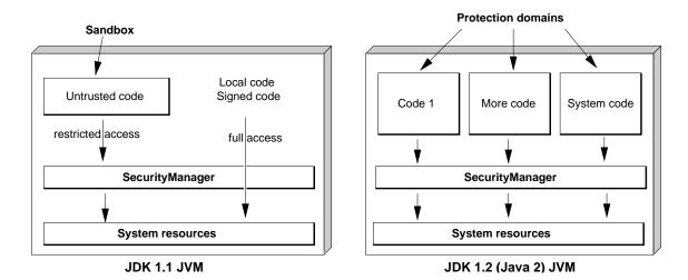
Figure 2.2: JDK 1.1 model (sandbox) and JDK 1.2 protection domains compared. In JDK 1.1 the code is either in the sandbox or trusted. In Java 2 the code is divided into different protection domains.
