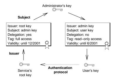
Figure 2.1: Simple SPKI certificate loop.
