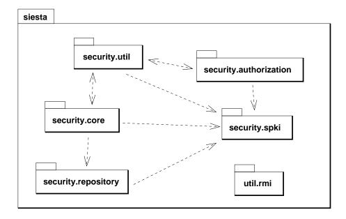
Figure 5.1: UML package diagram, also showing the dependencies between the packages. Some generic utility packages which are not essential for this discussion are not shown.
