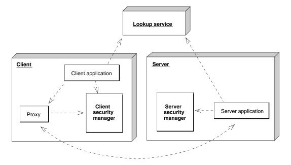
Figure 4.1: The parties and components involved in the architecture.
