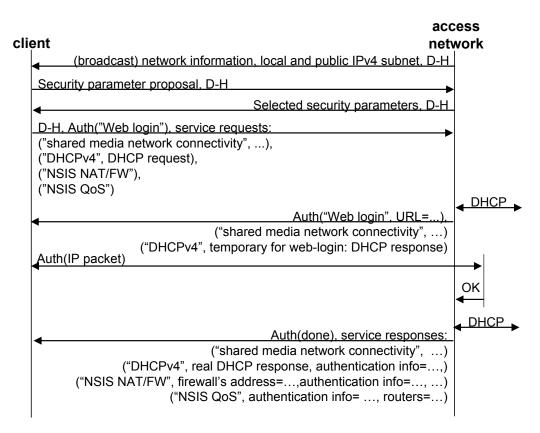
Fig. 3. NAP with IPv4 network attachment.
