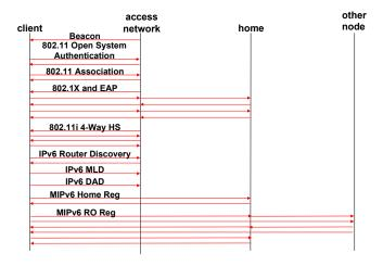
Fig. 1. IPv6 network attachment with existing protocols.
