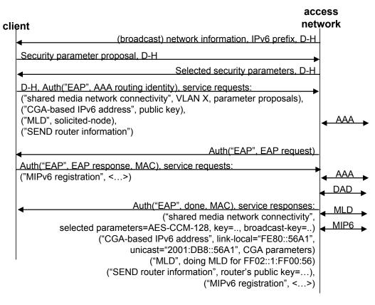
Fig. 2. NAP and IPv6 network attachment.
