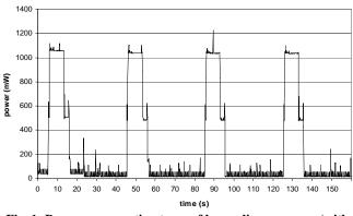
Fig. 1: Power consumption trace of keep-alive messages (with acknowledgment) in 3G with 40-second interval.
