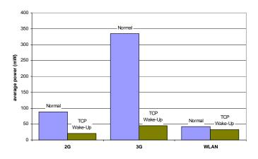
Fig. 8: Estimated power consumed by normal Mobile IPv4 NAT traversal (30-second UDP keep-alives) vs. TCP Wake-Up (600-second TCP keep-alives).
