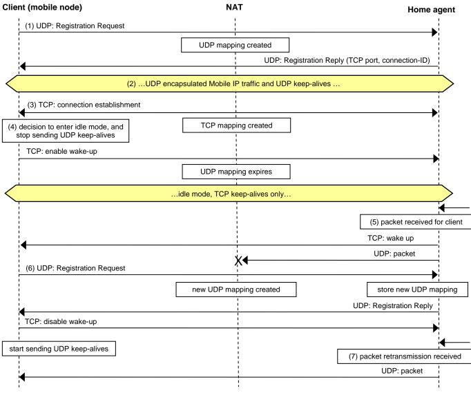
Fig. 7: Overview of TCP Wake-Up with Mobile IPv4.
