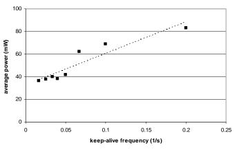
Fig. 6: Average Wireless LAN power consumption of keep-alive messages (with acknowledgment) with different intervals. The least-squares fitted line corresponds to 280 mJ/keep-alive plus 33 mW background consumption.
