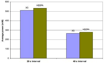
Fig. 5: Average power consumption of a keep-alive exchange (with acknowledgment) on Nokia N95, comparing 3G (without HSDPA) with HSDPA.
