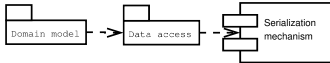
Figure 2.2: The Data-Access Objects Approach. The data access classes are directly coupled to the serialization mechanism, but reuse of domain classes may be possible.
