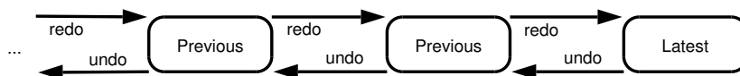
Figure 3.3: Linear Undo. The user can browse the history back and forth in a step-by-step manner.
