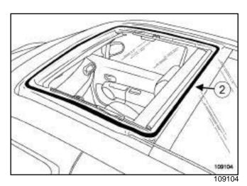
Desition the seal weld on the rear centre section (2).
