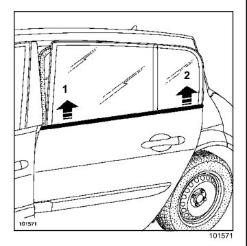
Unclip the exterior weatherstrip in the direction of (1) and (2) using tool (Car. 1363).
