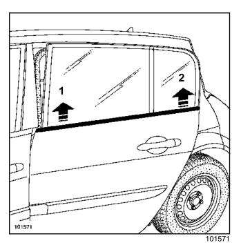
Carefully remove the weatherstrip in the direction of (1) and (2) using tool (Car. 1363).
