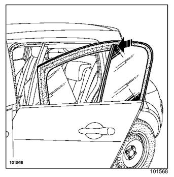
□ Remove the « seal and fixed window » assembly from the door.
