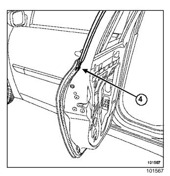
□ Unclip the upper clip from double seal (4).
