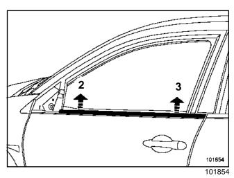
Carefully remove the weatherstrip in the direction of (2) and (3) using tool (Car. 1363).
