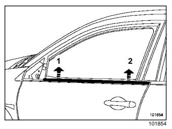
Carefully remove the weatherstrip in the direction of (1) and (2) using tool (Car. 1363).
