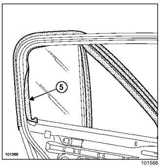
Offer up the « seal and fixed window » to the door.Clip in interior surface seal (5).
