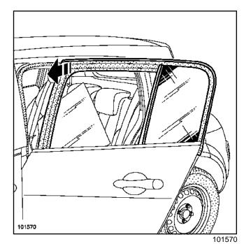
□ Unclip the front section of the seal.
